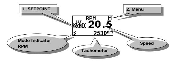
Operating in this mode is very similar to using the Wakeboard mode, except the system is now controlling to an RPM **SETPOINT**.
