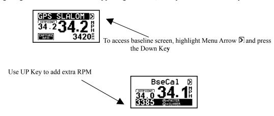
This screen example shows the RPM that was captured on this boat was 3385 for 34.0 mph. Because when you tow a skier additional RPM is required, we recommend you add 160 RPM to each of your captured baselines (ie. adjust for each speed setting). In this screen, we recommend you manually adjust it up to 3545 (3385 + 160). This tweak will allow for a quicker, more accurate engagement and control for course skiers.
