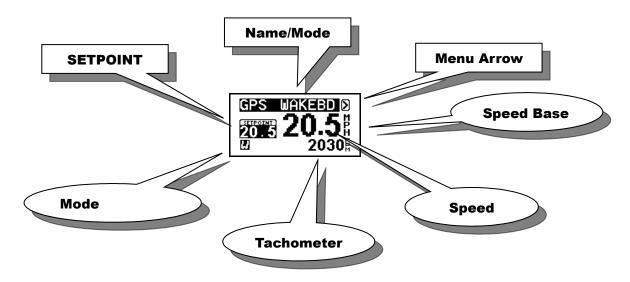
When system is ON, the screen will appear as above with set point speed at left. By using Menu Key you can move around the screen and highlight set point to make speed changes.
