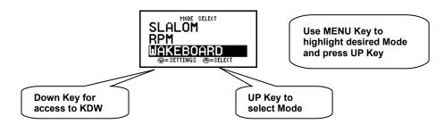
**KDW Adjustable Pull Parameter** – This background setting allows you to tailor the pull characteristics. To access, highlight Menu Key ∑, and press the DOWN Key to access this KDW screen:
