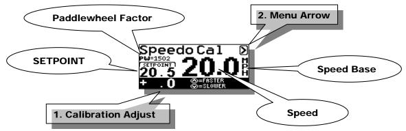
We recommend you check and calibrate if necessary at 20 mph.
