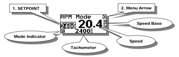
Operating in this mode is very similar to using the Wakeboard or Trick modes, except the system is now controlling to an RPM **SETPOINT**.
