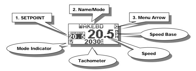
When system is ON, the screen will appear as above with set point speed at left. By using Menu Key you can move around the screen and highlight set point to make speed changes.
