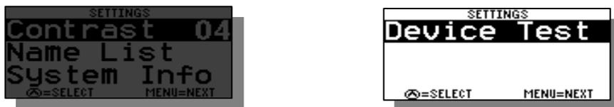
**Contrast** – To adjust the darkness of the lettering on the screen you can change the contrast. This value can be adjusted from 0-5 and is saved in the memory. The smaller the number, the brighter the screen will be in bright sun.
