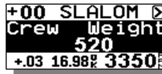
*Enter the Crew Weight in pounds using the UP and DOWN keys. Press the MENU key to confirm and continue.*
