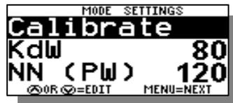
**Calibrate** – Used to calibrate the PerfectPass digital speedometer readout. The procedure for adjusting this can be found in the *Section 7: Digital Speedometer Calibrate*. The calibration screen can also be accessed from the Main WAKEBOARD Screen by pressing the **DOWN** key with the
