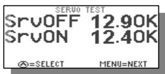
**SrvOFF 13.5 OK**– The system powers down the servo motor and measures the supply voltage level. The voltage with engine running should be in the range of 13 to 14 V. If the voltage is below 13.0 V, the display will show it as low (“LO”).
