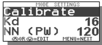
**Calibrate** – Used to calibrate the PerfectPass digital speedometer readout. The procedure for adjusting this can be found in the Digital Speedometer Calibrate Section 7, Page 19. The calibration screen can also be accessed from the Main Trick Screen by pressing the **DOWN** key with the
