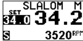
This mode allows you to set speeds in 2 mph increments ranging from 24 – 36 mph. It is designed for those wishing to use the system for open water skiing.
