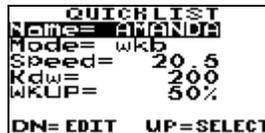
Scroll through the alphabet using **UP** & **DOWN** keys, and then press **MENU** to move to next position. Press the **MENU** key to move through the settings. You can even enter a rider's preferred wake plate position and KDW value.
