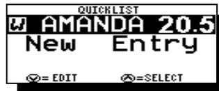
**Creating Names** – First enter the Quick List. Press the **MENU** key until [NEW ENTRY] is highlighted. Then press the **UP** key to enter a new name. The following screen will then appear:
