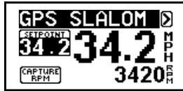
This mode allows you to set speeds in 2 mph increments ranging from 24 – 36 mph. It is designed for those wishing to use the system primarily for open water skiing.
