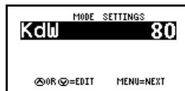
**KDW (Throttle Pull Rate)** – KDW can be changed using up or down keys. The higher the value, the more aggressive the control. Heavy boats may need higher values. Factory setting is about 90. Normal range is 50 – 150. (If this value is set too high, the control may become a little erratic and engagement may not be as smooth).
