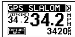
Use Menu Key to highlight the “Capture RPM”, then press UP Key and calibration is complete.
