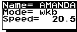
Scroll through the alphabet using **UP & DOWN** keys, and then press **MENU** to move to next position. Press the **MENU** key to move through the settings. If you are programming a JUMP or SLALOM name there will be another page of settings to enter.
