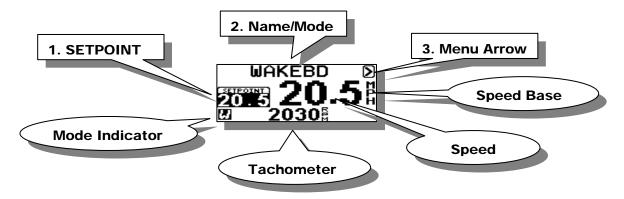
2. <u>RPM Mode</u> where the user sets an rpm value. Designed for higher speed use such as open water skiing or cruising.
